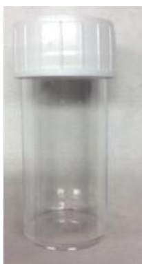
Use 50 mL plastic vessel for casting cement pastes
