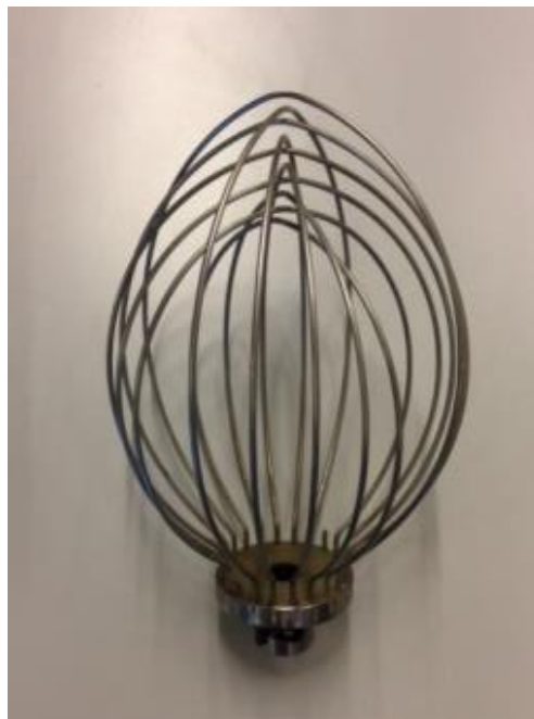
Blade to be used for preparing cement paste in accordance to EN 196-1 and EN 196-3
