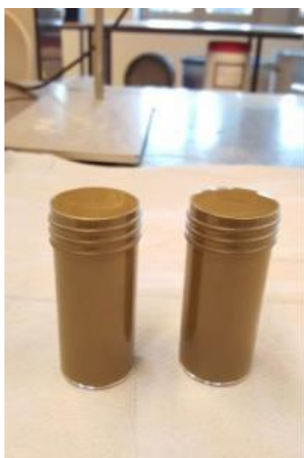
Cast cement paste in plastic vessels and fill it up
