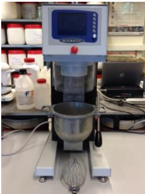
Mixer for preparing cement paste in accordance to EN 196-1 and EN 196-3
